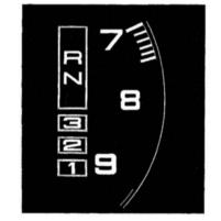
This display is on the instrument panel in the tachometer. It shows you the position of the shift lever (see p. 26).
