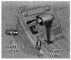
6. Remove the cigarette lighter from its socket and plug the power cord end into the socket. Make sure the key is in the ignition switch at Lock (0).
