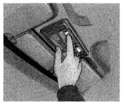
When the three position switch is at the center position with both doors closed, the two bulbs in the interior light can be turned on separately by the pushbutton switches next to them. Push the switch to turn the light on or off.
