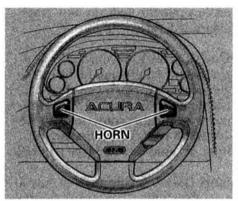
Press either of the buttons on the steering wheel spokes to sound the horn.
