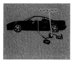
5. Place the air pump near the flat tire. Open the nearest window, and route the air pump's power cord through the open window.
