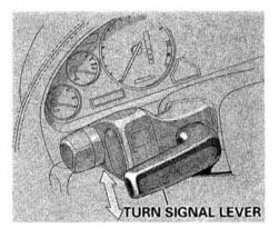
Signal a turn or lane change with this lever. Push down on the lever to signal a left turn, and up to signal a right turn. If you push it up or down all the way, the turn signal continues to blink even when you release the lever. It shuts off automatically as you complete the turn. To signal a lane change, push lightly on the turn signal lever in the proper direction and hold it. The lever will return to the center position as soon as you release it.
