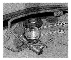
The fluid should be between the MIN and MAX marks on the side of the reservoir. If it is at or below the MIN mark, it is an indication that your brake system needs attention. Have the brake system inspected for leaks or worn brake pads. If you add brake fluid to bring it up to the MAX mark, use Genuine Honda Brake Fluid or an equivalent that is marked DOT3 or DOT4 only. Brake fluid marked DOT5 is not compatible with your car's braking system.
