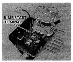
4. Connect one jumper cable to the positive (+) terminal on the booster battery. Connect the other end to the JUMP START terminal in the fuse box.
