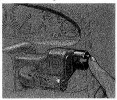
Push the large red button on the right pod to turn on the hazard warning lights (four-way flashers). This causes all four outside turn signals and both indicators in the instrument panel to flash. Use the hazard warning lights if you need to park in a dangerous area near heavy traffic, or if your car is disabled.
