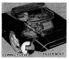
Check the oil level a couple of minutes after shutting off the engine with the car sitting level. Remove the transmission filler bolt (located next to the left axle). The oil level should be up to the edge of the bolt hole. Feel inside the bolt hole with your finger. If you do not feel any oil, slowly add oil until it starts to run out of the hole. Reinstall the filler bolt and tighten it securely. Only use an SF or SG grade motor oil, with a weight of 10W-30 or 10W-40.
