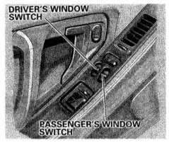
The driver's armrest has a master power window control panel. To open the passenger's window, push down on the switch and hold it down until the window reaches the desired position. To close the window, push up on the window switch. Release the switch when the window gets to the position you want. The master control panel also contains these extra features:
