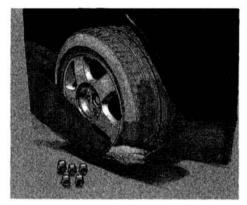
11. Remove the wheel nuts and flat tire.
