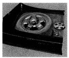
21. Store the jack, wheel wrench, extension, air pump, pressure gauge, screwdriver and flat tire in the trunk. Temporarily keep the wing bolt and center cap in the trunk as well. See **Replacing Tires** on page 155 for tire replacement. Storing the Folding Spare Tire Before returning the folding spare tire to its compartment, you must let out all the air. It will fold back to its original space saving shape.
