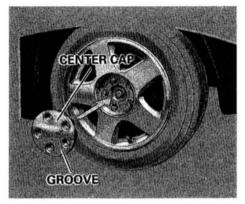
7. Install the center cap with the groove closest to the valve.
