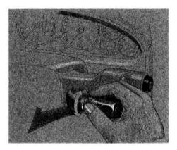
In intermittent, the wipers operate every few seconds. You can adjust this delay by turning the INT TIME ring on the lever. This allows you to vary how often the windshield wipers sweep when driving in light rain or snow. In low speed and high speed, the wipers run continuously.
