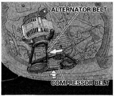
You should check the condition of the two engine belts every six months. Examine the edges of each belt for cracks or fraying. Check the tension of each belt by pushing on it at the point shown in the diagram. The belts should have the follwing "play" or deflection. Alternator belt: one-half in. (12-14 mm) Compressor belt: seven-sixteenths in. (10-12 mm)
