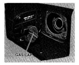
3. Remove the gas cap slowly. You may hear a hissing sound as pressure inside the tank escapes. Place the gas cap on the inside of the door as shown.
