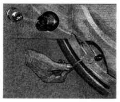
4. As the tire deflates, it will fold back to its original shape. When the air stops coming out of the tire, use the notch on the valve cap to tighten the valve core.
