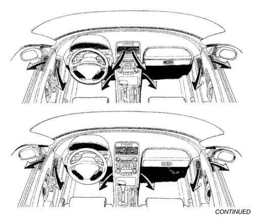
The main air flow is divided between the floor vents and windshield defroster vents.
