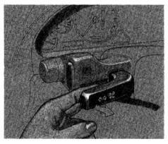
To change between low beams and high beams, pull back on the turn signal lever as far as it will move towards you, then let go. The high beam indicator will light (see page 26). To flash the high beams when the headlight doors are closed, pull back and hold the turn signal lever. This simultaneously raises the headlight doors and turns on the high beams. Release the lever and the high beams go off. Within a few seconds, the headlight doors will close automatically.
