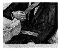
4. Make sure the seat belt is not twisted. Pull up on the shoulder belt to remove any slack. Place the shoulder belt across your chest and over your collarbone, not under your arm.
