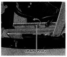
4. Remove the drain plug from the bottom of the radiator.
