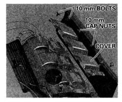
Replace the spark plugs one side at a time. Make sure the front cylinder spark plug caps and the backside of the cover have the letter "FR" on them and the rear cylinder spark plugs and the backside of the cover have "RR". To replace them:
