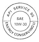
The numbers in the middle tell you the oil's SAE viscosity or weight. Select the oil for your car according to this chart:
