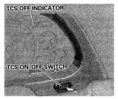
This switch is on the dashboard behind the right control pod. It lets you turn the Traction Control System on and off. You cannot turn off the TCS while the TCS Activation light is flashing. Deactivate the system by pressing the TCS On/Off switch. The light in the switch goes out, and the TCS OFF indicator comes on. Pressing the switch again turns the system back on.
