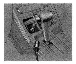
17. When finished, reach in and turn the ignition switch to Lock (0). Unplug the air pump power cord.
