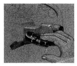
To operate the wipers in mist mode, push the control lever down. The wipers run at high speed until you release the lever. This gives you a quick way to clear the windshield.
