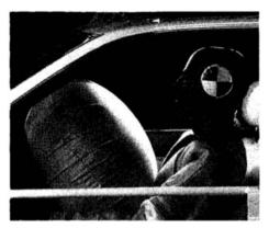
The SRS is designed to activate if the car is involved in a frontal collision at road speeds. The airbag cushions the driver's face and chest, while the knee bolster helps prevent the driver from sliding under the dashboard while helping to protect the driver's knees. The SRS will not protect the driver in a side impact, rear impact, or roll-over collision. The driver and passenger should wear their seat belts at all times for maximum protection.
