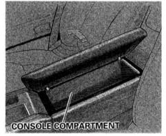
To open the console compartment, lift the left edge.
