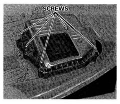
3. Loosen the six phillips-head screws around the edge of the cover. Remove the cover and set it aside.
