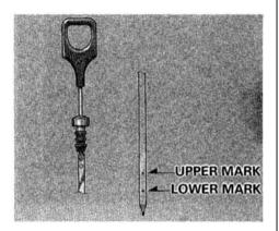
4. Remove it again and check the level.It should be between the upper and lower marks.
