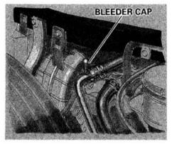
10. Remove the bleeder cap from the top of the heater inlet.
