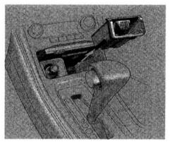
Open the ashtray by lifting the lid up. To close the ashtray, push the lid down. To remove it for emptying, lift the lid up to the open position, and push it up further. The ashtray will pop out slightly so you can grasp it and pull it all the way out. After emptying, push it all the way back in.
