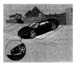
Curbs and steep inclines could damage the front and rear bumpers. Low curbs that do not affect the average sedan may be high enough to hit the bumper on your NSX. The front or rear bumper may scrape when trying to drive onto an incline, such as a steep driveway or trailer ramps. • Because of the low-profile tires fitted to your car, the alloy wheels are closer to the ground. Driving over a pothole or road debris at too high a speed can seriously damage a wheel. Slow down under these conditions.
