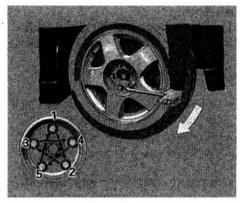
6. Remove the folding spare tire and install the original tire and wheel nuts. Lower the car and tighten the wheel nuts securely in a criss-cross pattern. Tighten to:
