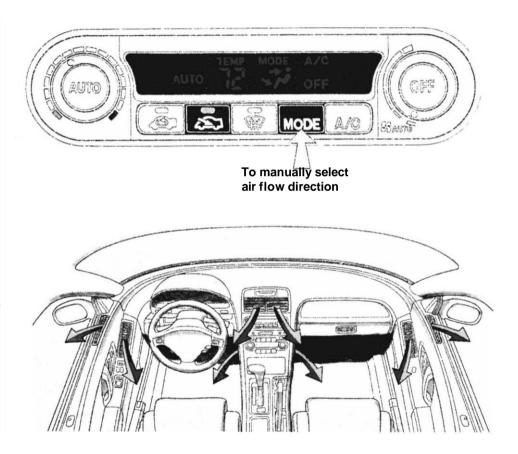
The main air flow is divided between the dashboard/door vents and the floor vents.
