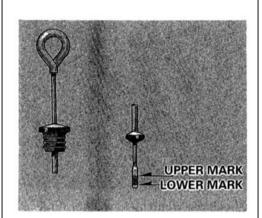
4. Check the fluid level. It should be between the upper and lower marks.
