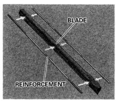
5. Examine the new wiper blades. If they have no plastic or metal reinforcement along the back edge, remove the metal reinforcement strips from the old wiper blade and install them in the slots along the edge of the new blade.
