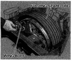
3. Open the hood (see page 97). Unscrew the wing bolt holding the folding spare tire. Remove the folding spare tire from the compartment. The wing bolt and wheel may be very warm from the air passing through the radiator. Use a cloth or gloves (not provided) to protect your hands when removing the spare tire.
