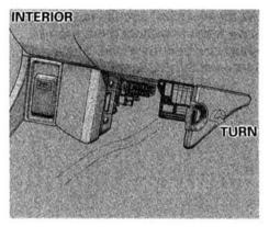
The interior fuse box is underneath the dashboard on the driver's side. To open, turn the knob as shown.
