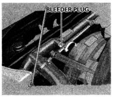
5. Loosen the bleeder plug on top of the radiator.
