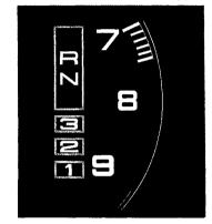
An indicator in the tachometer shows which shift position you are in.
