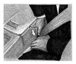
To unlatch the seat belt, push the red PRESS button on the buckle. The seat belt will retract out of your way. If it doesn't, pull it out and check for twists or kinks in the belt.
