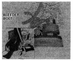
11. Loosen the bleeder bolt on top of the engine.
