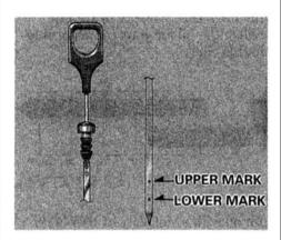
3. Pull the dipstick out and look at the oil level at the end of the dipstick. If it is between the upper and lower marks, the level is correct.
