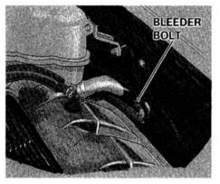
12. Loosen the bleeder bolt near the expansion tank.
