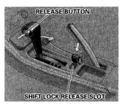
4. Push down on the key while you press the release button and move the shift lever out of Park to Neutral.
