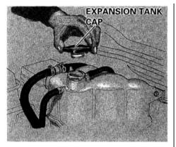
14. Fill the expansion tank to about 1 inch above the MAX line. Put the cap back on the tank, only tighten it to the first stop. Start the engine and let it run until it warms up (the radiator cooling fan comes on at least twice). 15. Turn off the engine. Check the expansion tank and, if needed, add coolant to bring it up to the MAX line. Tighten the expansion tank cap. Reinstall the cover on the car's underside.
