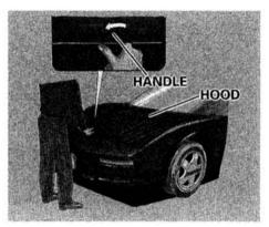
Standing in front of the car, put your fingers under the front edge of the hood to the right of center. Slide your hand to the left until you feel the hood latch handle. Push this handle to the left until it releases the hood. Lift the hood.
