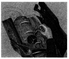
6. Put the new spark plug into the socket, then thread it into the hole. Screw it in by hand so you do not crossthread it.
