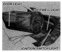
When you open the driver's door, lights for the driver's footwell and the ignition switch turn on to assist you. These lights stay on for a few seconds after you close the door.
