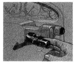
To clean the windshield, pull back on the wiper control. The washers spray until you release the lever. The wipers run at low speed while you're pulling the lever, then complete one more sweep of the windshield after you release it.
