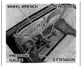
4. Open the trunk (see page 42). Lift the cover; remove the jack, wheel wrench, extension, air pump, pressure gauge and screwdriver from the trunk. The tools may become very hot while the car is being driven. Wear gloves or use a protective cloth when handling the tools.
