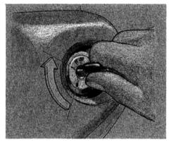
Reach into the car and turn the ignition switch to Accessory (I). This will start the air pump to inflate the tire.
