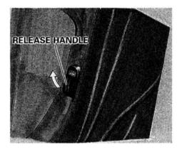
1. Locate the release handle on the rear of the driver's door opening, next to the seat. Pivot this handle towards the driver's seat. The rear window will pop up slightly.
