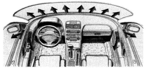
If there is frost on the windows, first select the (a) position. If the windows are fogged, select the aposition. Warmed air will then flow from the windshield and side defroster vents.
