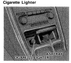
The ignition switch must be in Accessory or ON for the cigarette lighter to work. To heat up the lighter, push it in. It will pop out when it is ready for use. Do not hold the lighter in while it is heating up, you could cause it to overheat. Ashtray
