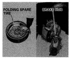
12. Before you put on the folding spare tire, wipe any dirt off the mounting surface of the brake hub and the wheel. This will assure a tight, even contact between the wheel and hub.
