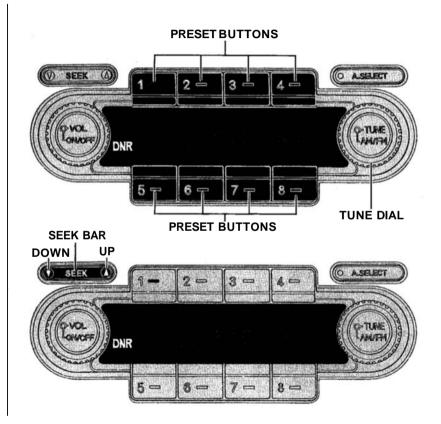
The A. SELECT function allows you to find stations easily when you are in an unfamiliar area. Press the A. SELECT button. The system automatically scans both the AM and FM bands, memorizes the eight strongest stations on each band, and stores them in the eight preset buttons. You can then use the buttons to tune to those stations. The light in the A. SELECT button stays on as a reminder. You cannot manually change any presets with A. SELECT on.
