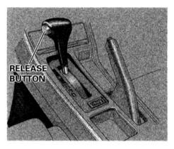
The shift lever has seven positions. It must be in Park or Neutral to start the engine.
