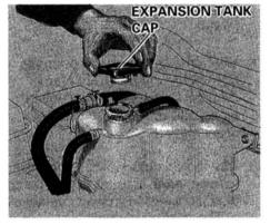
3. With the engine and radiator cool to the touch, remove the expansion tank cap.
