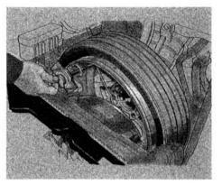
8. Store the folding spare tire in the front compartment with the outside surface of the wheel contacting the bracket of the spare tire well. Securely tighten the wing bolt.
