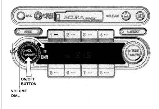
Select the AM or FM band by pushing the AM/FM button. The selected band is shown next to the frequency display.
