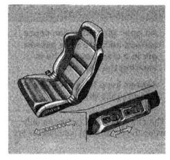
The power seats in your car are adjusted with the two switches on the outside of the seat bottom.
