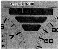
If the TCS develops a problem, the TCS indicator comes on and the TCS is automatically disabled. The TCS OFF indicator does not come on under this condition. If you see this, pull to the side of the road at your first opportunity and turn off the engine. Reset the system by restarting the engine, and see if the TCS indicator goes out. If it remains on, or comes back on again while driving, have the TCS inspected by your Acura dealer. You can still drive the car without TCS.
