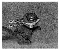
Check the fluid level in this reservoir after driving the car for at least a few minutes. It should be between the MIN and MAX marks on the side of the reservoir. If it is at or below the MIN mark, it may indicate a problem in the braking system. Have the dealer inspect your car. If the fluid level is half an inch or more above the MAX mark, it may indicate a problem in the Anti-lock brake system. Have your dealer inspect the system as soon as possible.
