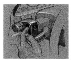
Pressing the Cruise Control Master Switch turns the system completely off. This erases the previous cruising speed from memory. To use the system again, you must set the system up as explained in **Using the Cruise Control.**  Horn
