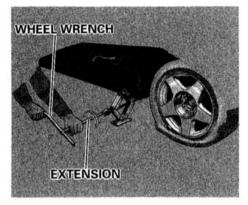
10. Use the extension and wheel wrench as shown to raise the car until the flat tire is off the ground.
