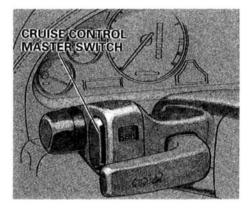
The switch on the left pod is the cruise control master switch. For instruction on using the cruise control (see page 36).
