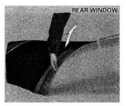
2. Stand just behind the driver's door. Reach under the rear edge of the rear window at its center and raise it. It will stay up by itself.
