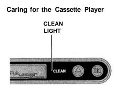
The cassette drive picks up dirt and oxides whenever you play a tape. This builds up over time and causes the sound quality to degrade. To prevent this, you should clean the cassette drive after every 30 hours of use. Your dealer has a cleaning kit available for this purpose. After 50 hours of use, the CLEAN light comes on to remind you to clean the cassette drive. After cleaning the drive, turn off the CLEAN light by pushing it in with the tip of a ballpoint pen or similar object.
