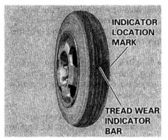
The folding spare tire has a shorter tread Me than a regular tire. Replace it when you can see the tread wear indicator bars. The spare tire is not designed to be mounted on a regular wheel, and the compact wheel is not designed for mounting a regular tire. Diagnosing why your engine won't start falls into two areas, depending on what you hear when you turn the key to START(III):
