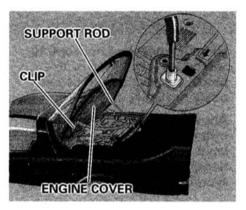
3. Lift the engine cover. Pull the support rod out of its clip on the engine cover and insert the end into the square hole in the bracket.
