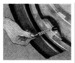
18. Screw the valve cap on the valve tightly with your hands.
