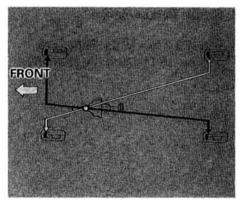
If this happens, you will immediately notice that the brake pedal goes down much farther and you need to press on it much harder. A much longer distance will be needed to stop the car.
