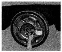
13. Put on the folding spare tire with the air valve toward the bottom. Put the wheel nuts back on fingertight, then tighten them in a crisscross pattern with the wheel wrench so the wheel is firmly against the hub. Do not try to tighten them fully. Inflate the folding spare tire only when it is on the car. Inflating it while it is lying on the ground may trap stones or other foreign matter between the tire and the wheel rim.
