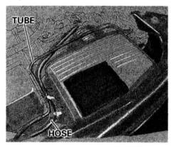
The air filter is inside the box on the driver's side of the engine compartment. To replace it:
