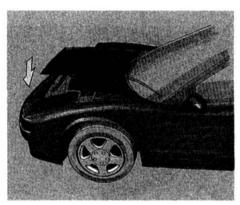
6. To close the hood, lower the hood about halfway down and let the hood drop. Make sure the hood is securely latched.
