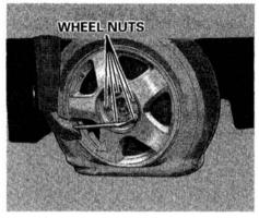
8. Loosen the five wheel nuts 1/2 turn with the wheel wrench.
