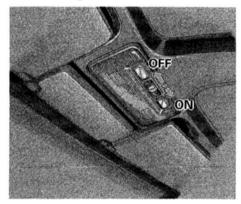
The interior light, on the ceiling between the sun visors, has a threeposition switch. With the switch in the OFF position (far left), the light will not come on. In the center position, the interior light comes on when you open either door. In the ON position (far right), the interior light is on all the time.
