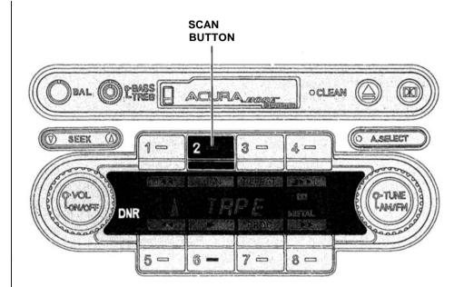
The ►, and SCAN functions use silent periods on the tape to find the end of a selection. These features may not work satisfactorily on tapes that have almost no gap between songs, a high noise level between songs, or silent periods in the middle of songs.
