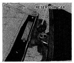
Check the windshield washer fluid level as follows:
