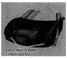
Periodically check the engine's radiator and air conditioning condensers (located in the openings below the parking lights) for leaves, insects, and dirt stuck to the front surface. These block the air flow and reduce cooling efficiency. Use a light spray from a hose or a soft brush to remove them.
