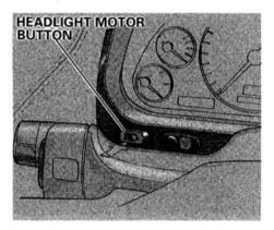
To raise and lower the headlight doors without turning them on, push the dashboard button behind the left pod.
