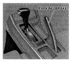
To apply the parking brake, pull the lever up fully. To release it, pull up slightly, push the button, and lower the lever. The parking brake light on the instrument panel should go out when the parking brake is fully released (see page 23). If you try to drive the car without releasing the parking brake, the Anti-lock brake system cannot work properly, and the rear brakes can be damaged.
