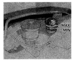
The fluid should be between the MIN and MAX marks on the side of the reservoir. If it is not, add brake fluid to bring it up to that level. Use the same DOT3 or DOT4 brake fluid specified for the brake system.
