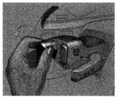
The rotating switch on the left pod controls the headlights. Turning this switch to the first position "•" turns on the parking lights, tail lights, instrument panel lights, side-marker light, and rear license plate lights. Turning the switch to the second position "•" raises the headlights and turns them on. If you leave the lights on with the ignition switch in Accessory or Lock, you will hear a reminder chime when you open the door.
