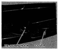
For very short distances such as freeing the car, you can use the tiedown hook on the lower right of the front bumper. Remove the cover to expose the hook. This hook is not for open-road towing (see **Towing**, page 202). If your car needs to be towed, call a professional towing service or, if you belong to one, an organization that provides roadside assistance. Never tow your car behind another car with just a rope or chain. It is very dangerous.
