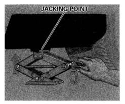
9. Locate the jacking point nearest the wheel you are removing by finding the arrow on the side of the body. Place the jack under the jacking point, then raise it by hand by turning the end bracket clockwise. Make sure the top of the jack fits exactly into the jacking point.
