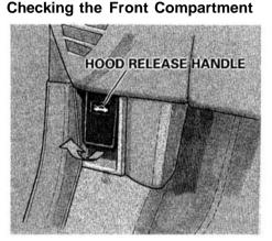
1. Pull the hood release handle, located under the left lower corner of the dashboard. Shift to Park or Neutral and set the parking brake.
