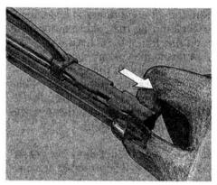
4. Remove the blade from its holder by grasping the tabbed end of the blade. Pull firmly until the tabs come out of the holder.
