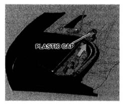
3. Remove the plastic cap on top of the headlight motor.
