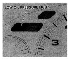
The oil pressure warning light should never come on when the engine is running. If this warning light comes on with the engine running, take immediate action.
