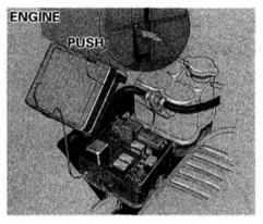
The engine compartment fuse box is located next to the air cleaner box. To open, push the tab as shown.
