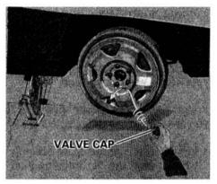
5. Put the rubber cap back on the valve cap. Screw the valve cap back on the folding spare tire valve.
