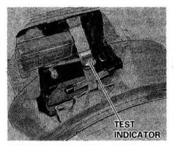
The electrolyte level should be between the two lines on the side of the battery. Low electrolyte level can be an indication of a problem with your car's charging system. Take the car to your dealer for service. Look through the test indicator window on the battery and check the indicator:
