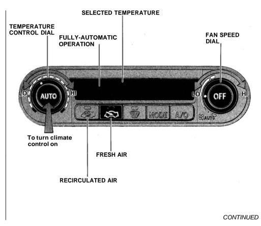
To heat or cool the interior faster, rotate the temperature control dial to its lower limit (60°F) or upper limit (90°F). The system then runs continuously at maximum cooling or heating. When the dial is set anywhere else within its range (61°F to 89°F), the system regulates the interior temperature to that value.
