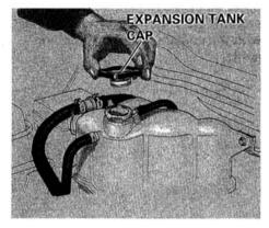
Loosen the expansion tank cap by turning it counterclockwise, without pushing it down, until it stops. This will relieve any remaining pressure in the cooling system. Then remove the cap by pushing down and turning. Fill the expansion tank with coolant to the MAX line and put the cap back on.
