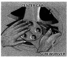
7. Remove the center cap from the wheel with the screwdriver. Use a cloth as shown to protect the cap and wheel.
