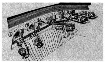
The bulbs for the taillights, brake lights rear, turn signals, and back-up lights are reached by pulling down the rear trunk liner.
