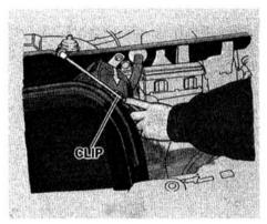
5. Snap the support rod back into its holding clip.
