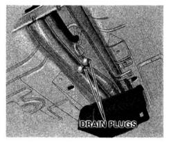
6. Remove the drain plugs from the coolant pipes under the car.
