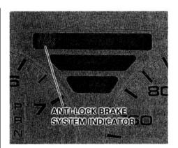
The Anti-lock brake system is selfchecking. If anything goes wrong, the Anti-lock brake system indicator on the instrument panel comes on (see page 24). This means the Antilock function of the braking system has shut down. The brakes still work like a conventional system providing normal stopping ability. You should have the dealer inspect your car as soon as possible.
