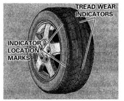
Your car's tires have wear indicators molded into the tread. When the tread wears down to that point, you will see a 1/2 inch wide band running across the tread. This shows there is less than 1/16 inch of tread left on the tire. A tire that is this worn gives very little traction on wet roads. You should replace the tire if you can see the tread wear indicator in three or more places around the tire.
