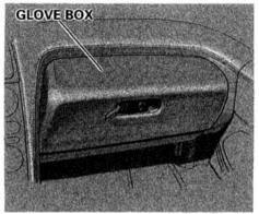
Open the glove box by squeezing the handle. Close it with a firm push. Lock or unlock the glove box with the master key.
