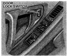
Each door has a door lock switch. Either switch locks both doors. Push LOCK to lock both doors, and the top portion of the switch to unlock them.
