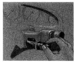
The lever on the right pod controls the windshield wipers and washers. The rotary switch at the end of the lever has three positions: INT—intermittent LO—low speed HI—high speed
