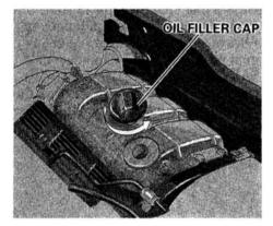
If the oil level reaches the lower mark on the dipstick, add one quart of the recommended engine oil. To do this, unscrew and remove the oil filler cap on top of the front valve cover. Pour in the oil, and replace the filler cap. Make sure it is securely tightened.
