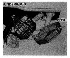
The underhood fuse box is located on the passenger's side of the front compartment. To open, push the tab as shown.
