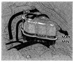
Look at the coolant level in the expansion tank. Make sure it is between MAX and MIN.If it is below the MIN mark, see **Adding Coolant** on page 131 for information on adding the proper coolant.
