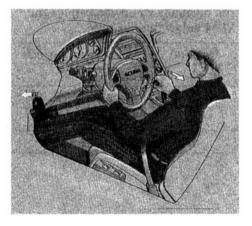
You must also press the release button to shift into Park. To avoid transmission damage, come to a complete stop before shifting into Park. The shift lever must be in Park before you can remove the key from the ignition switch.
