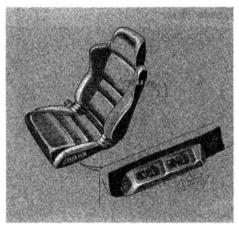
Adjust the seat-back angle by pushing the rear switch in the direction you want to move. You can adjust the seats with the ignition switch in any position. Adjust the seat position before you start driving.
