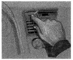
The digital clock displays the time with the ignition switch ON. To see the time with the ignition off, press and hold the DISPLAY button.
