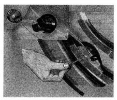
3. Remove the rubber cover on top of the valve cap. Use the notch on the valve cap to unscrew the spare tire valve core until the air starts coming out.
