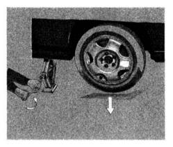
19. Lower the car to the ground and remove the jack.
