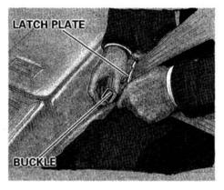
3. Pull the latch plate across your hips and snap it into the nearest buckle. Tug on the latch plate to make sure it is securely locked.
