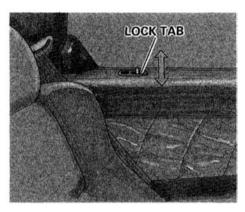
Each door also has a lock tab on the top. When you push down the lock tab on the driver's door, both doors lock. The lock tab on the passenger's door only locks that door. To get out of the car, pull each lock tab up or use the door lock switch before you open either door. The doors can be locked and unlocked from the outside with the key. Both doors lock when you use the key to lock the driver's door.
