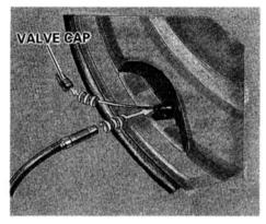
14. Unscrew the valve cap from the folding spare tire's air valve by turning it counterclockwise. Then screw on the air pump hose.
