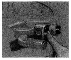
The rear window defogger will clear fog, frost, and thin ice from the window. Push the defogger button to turn it on and off. The light on the front of the pod lights to show the defogger is on. If you do not turn it off, the defogger will shut itself off after about 25 minutes. It also shuts off when you turn off the ignition. You have to turn it on again when you restart the car.
