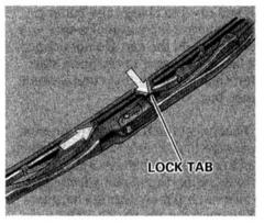
3. Disconnect the blade assembly from the wiper arm by pushing in the lock tab. Hold it in while you push the blade assembly toward the base of the arm. Gently lower the wiper arm against the windshield.
